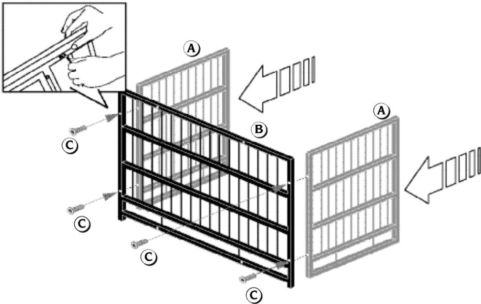
2. Attach Front Wall with door (D) to the Side Walls (A) with bottom tabs facing inward using four Hex Head Screws (C).
